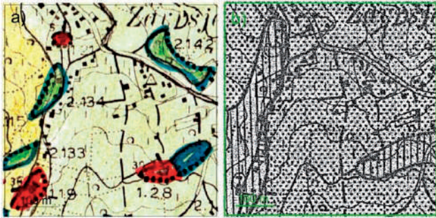
Figure 3 Segments of landslide maps from the study 'Lithology and categorization according to slope stability of Medvednica Mt. hills at the area of the Zagreb City' (Polak et al. 1979) for the area of Završje: a) lithological map in the original scale 1:10,000 with portray of landslides of which three are active (landslides no. 1,19, 1,21, 1,28), and three are inactive (landslides no. 2,133, 2,134, 2,142); and b) landslide susceptibility map in the original scale 1:10,000. A dotted area is category II – moderately stable slopes; and stripped areas is category III – moderately unstable slopes.
