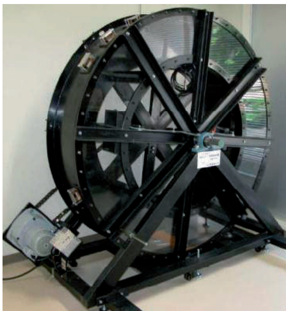
Figure 1 Photo of the apparatus to simulate a submarine landslide and damage of a communication cable.
