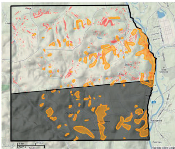
Figure 4 Model HA(ii). Shaded area represents the training split, orange polygons represent the landslides defined by the inventory, and red polygons represent the SVM-predicted landslides (source GoogleMaps).
