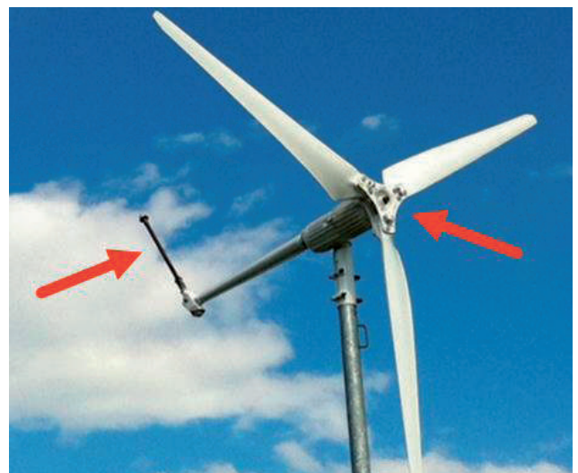
Figure 6 Damages on the windmill caused by bora. Red arrows are showing the damaged wind tail vane and head of the rotor.
