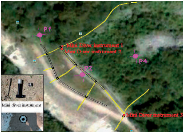
Figure 2 Positions of the Mini Diver instruments near the foot of the Grohovo landslide.
