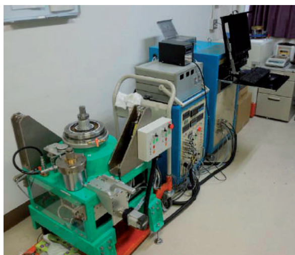
Figure 1 Transportable Ring Shear Apparatus, ICL-1 with its Instrument box, Monitoring box and Control box.
