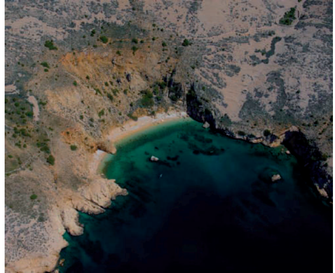
Figure 9 Debris avalanche provoked by marine erosion: the southeastern coast of the Island of Krk (Photo: Ž. Gržančić).
