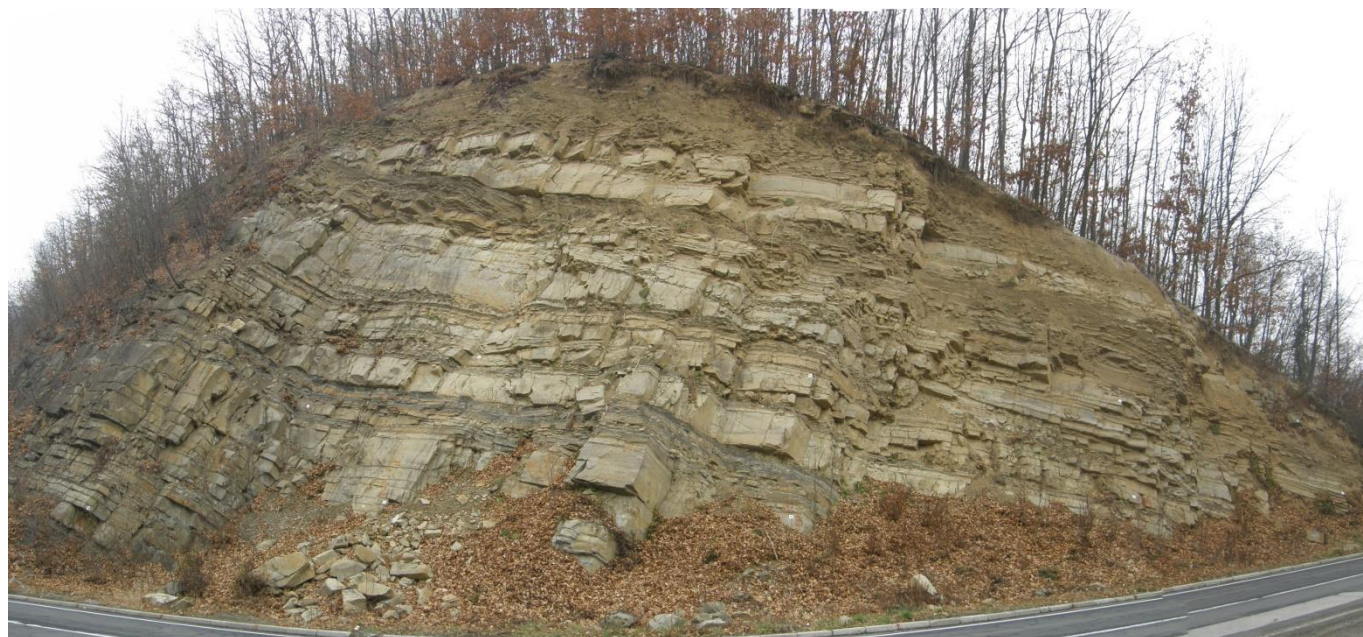
Figure 2 Panoramic view of the rock slope of interest near Ljig (approximate dimensions 60x30m), brighter light-grey parties are sand-stone strata, while less competent parties are dark-greyed (photo B. Abolmasov).
