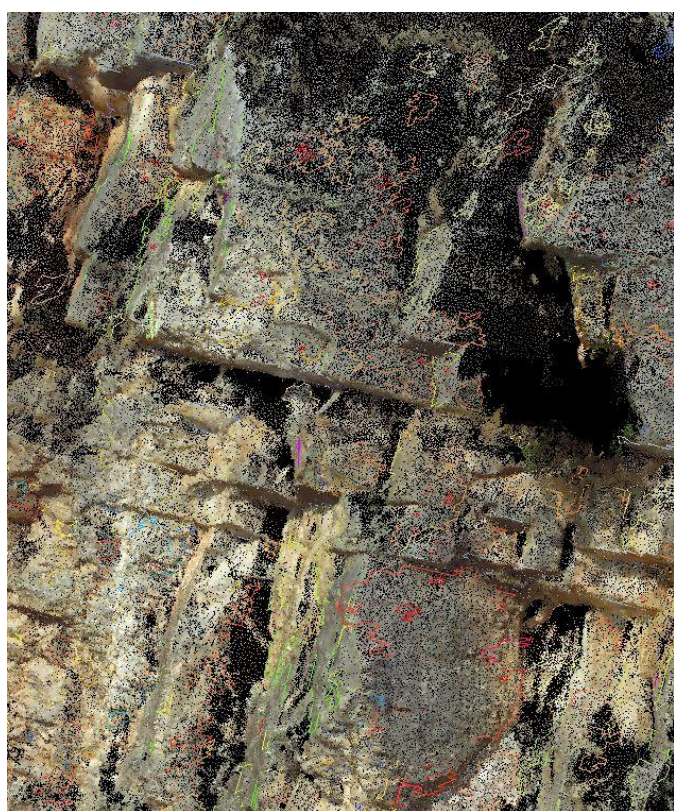
Figure 3 Automatically generated patches plotted on the point cloud in Split-FX software.
