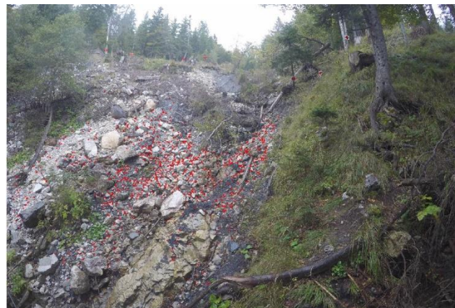
Figure 6 Detected target positions (red pluses) and well-defined points on the landslide (red dots).
