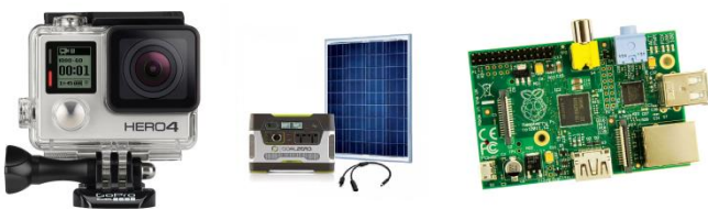
Figure 1 Hardware used to determine daily displacements – 2 GoPro cameras, a photovoltaic panel, and a Raspberry Pi miniature computer.
