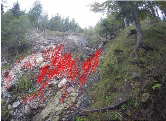
Figure 8 2D displacements of signalized targets (blue) and 2D displacements points of interest on the landslide (red). (All displacements are enlarged by a factor of 20x).
