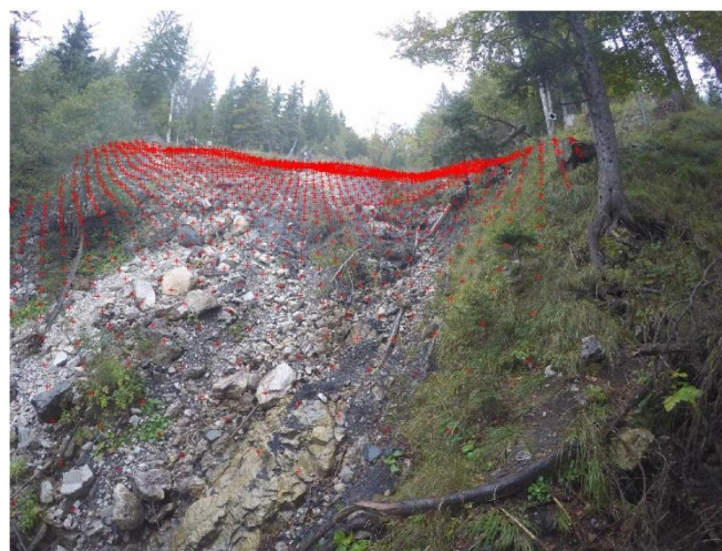
Figure 7 Digital terrain model projected on camera view.
