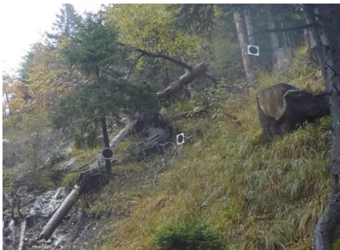
Figure 5 Subset of image from Figure 4 showing positions of photogrammetric targets using a Harris corner detector to detect well-defined points of interest on the landslide.
