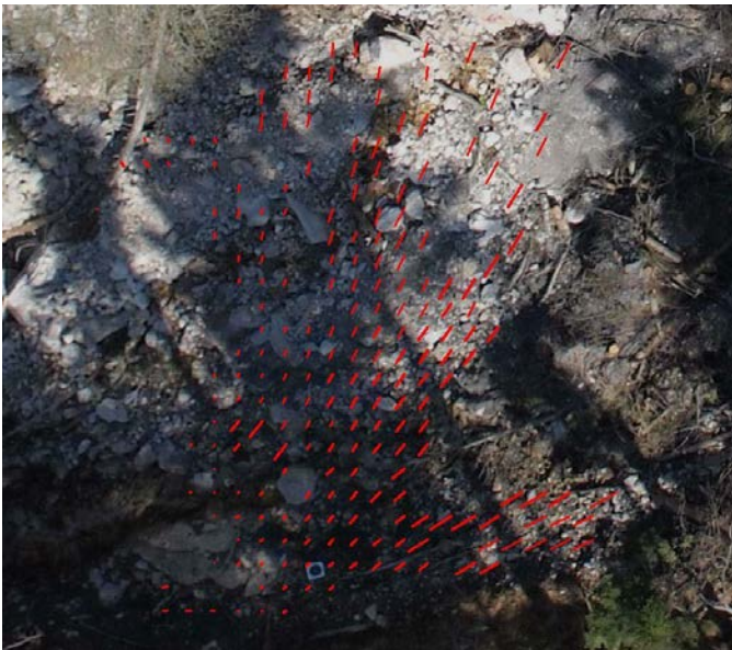
Figure 9 3D regular grid of landslide displacements displayed over the orthophoto map.
