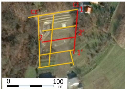
Figure 10 Landslide covered by GPR grid.
