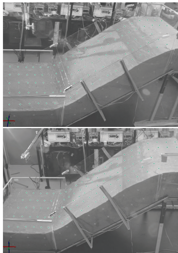
Figure 3 Left-camera (top) and right-camera (bottom) view of the model with monitored points (green dots) (from Maksimović (2020), Pajalić et al. (2021)).
