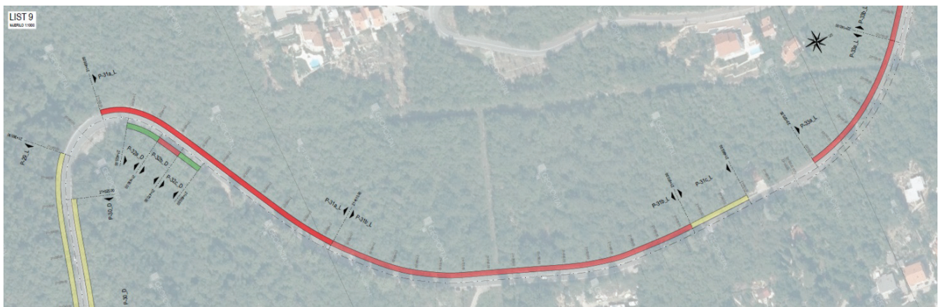
Figure 5 Distribution of the priority protection groups from km 21+240 to km 22+160; Group C (red line), Group B (yellow line) and Group A (green line).
