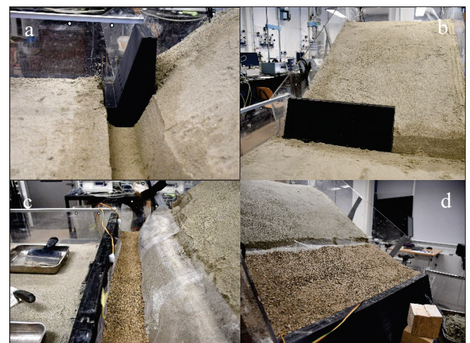
Figure 3 Installation of gravity wall and buttressing embankment behind the wall in prepared sandy slope: a) excavated foundation pit and installed element of the gravity wall, b) a view at the partially installed wall in the foot of the slope, c) filling the gravel material behind the wall with installed sensors; geotextile is laid to the steps in the sandy slope; d) filled buttressing embankment behind the gravity wall along the slope.
