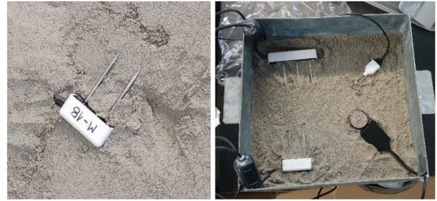
Figure 5 Installation of TEROS 10 during model build-up (left) and calibration for clean sand.
