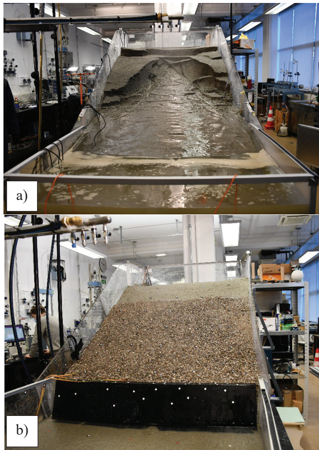
Figure 6 a) retrogressive slide in the test on the sandy slope without applied gravity wall after 120 min of rainfall; b) a view at the sandy slope with applied gravity wall after 120 min of rainfall.
