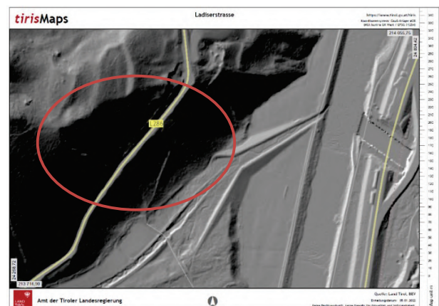
Figure 3 Close up of the digital terrain model, where the red ring indicates the Ladiserstrasse landslide area in 2018 (tirisiMaps 2014).
