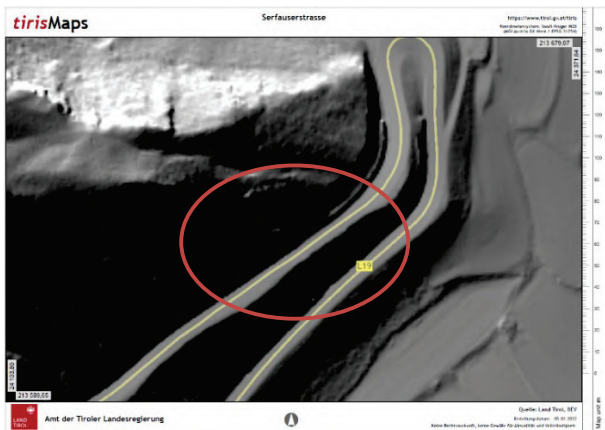
Figure 6 Detail of the digital terrain map showing unstable slope features, with the ring indicating the slope failure of the Serfauterstrasse in winter 2018 (tirisiMaps 2014).
