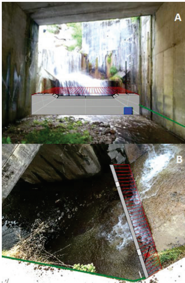
Figure 5 Design of the intercepting structure: A view from downstream, below the road bridge; B view from above.
