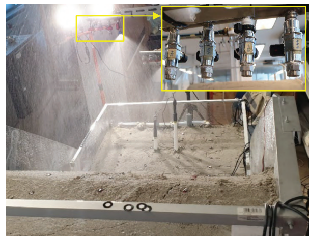
Figure 2 Simulated rainfall with an intensity of 23 mm/h with a detail of the sprinkler branch with axial flow full-cone nozzles.
